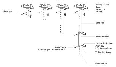
3 Use the appropriate number of screws for the projector size to attach the projector to the ceiling mount bracket.
